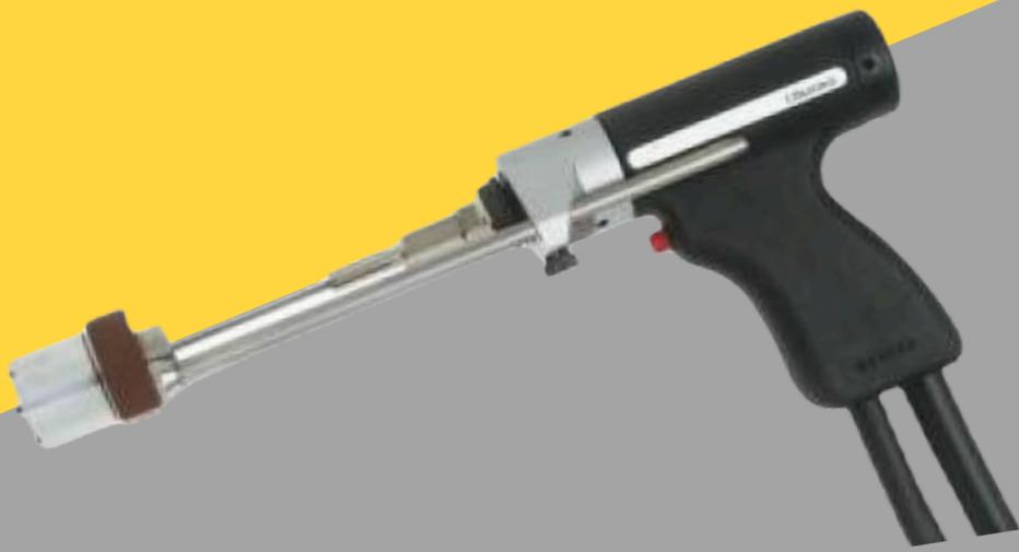
*The PSI 500 gun is a compact, durable tool designed for welding pins ranging from diameter 3 to 12. Equipped with an automatic length compensation system, it ensures consistent welding quality regardless of pin length or surface conditions. Its robust, high-quality mechanical components guarantee long-lasting performance, even under heavy-duty usage.*
