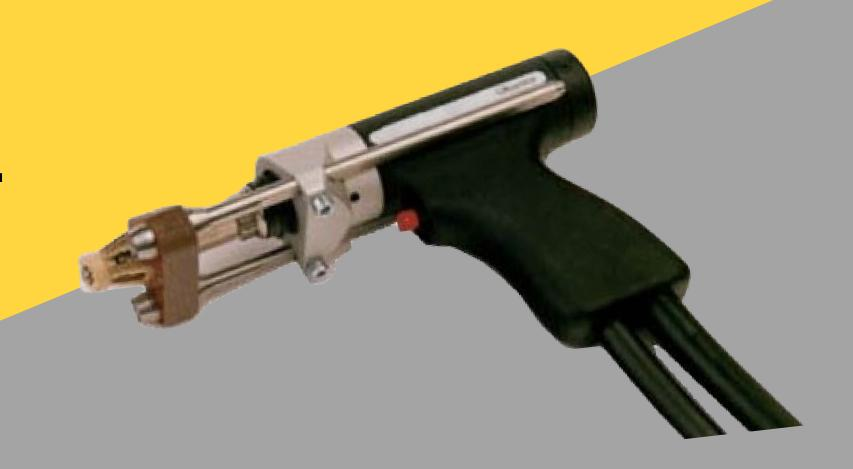
The PBI 500 gun is a compact and sturdy welding tool designed for studs with diameters from M3 to M12. It supports the use of ceramic rings in compliance with DIN EN ISO 13 918. Featuring an automatic length compensation system, the gun delivers consistent welding quality irrespective of stud length or surface conditions. Built with high-quality, durable mechanical components, it ensures reliable performance even under intensive use.
