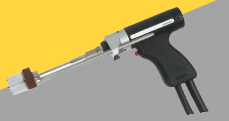
The PSI 500 gun is a compact, durable tool designed for welding pins ranging from diameter 3 to 12. Equipped with an automatic length compensation system, it ensures consistent welding quality regardless of pin length or surface conditions. Its robust, high-quality mechanical components guarantee long-lasting performance, even under heavy-duty usage.
