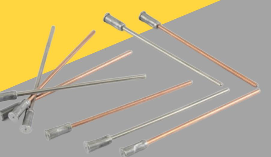
VBS bi-metal insulating pins are specifically designed for securing technical insulation to aluminum structures. Utilizing our new crimping technology, these pins provide enhanced durability and resistance to various loads, ensuring long-term fastening stability. For optimal performance, it is recommended to weld VBS pins using our N-5 capacitor welder or our INVERTER 500 welder.
