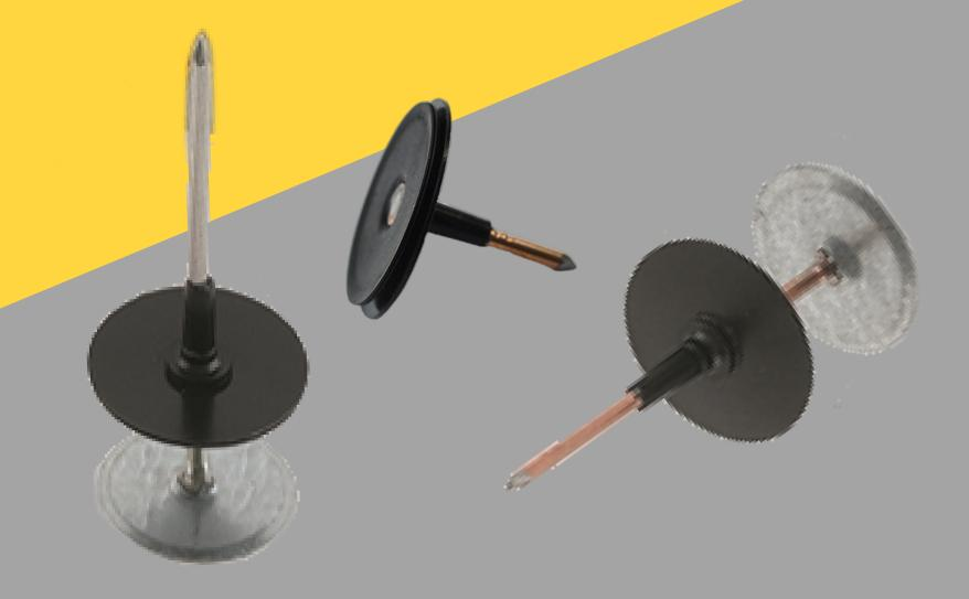
GZONI pins are engineered for the contact welding of technical insulation onto ventilation ducts and steel structures using the "reverse" welding method. These nails feature insulation on both the plate and the pin, preventing burn-through of the aluminum foil during welding. Before installation, an black insulator must be applied to the pin.
