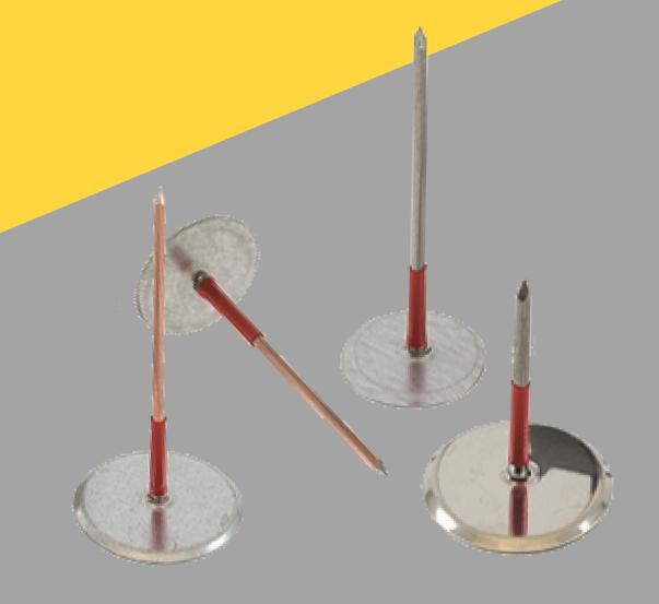
GZONI K pins are specially designed for welding technical insulation onto ventilation ducts and steel structures. These nails have insulation solely on the pin. For optimal results, it is recommended to use a spacer nozzle to create a gap between the aluminum foil and the pin plate.
