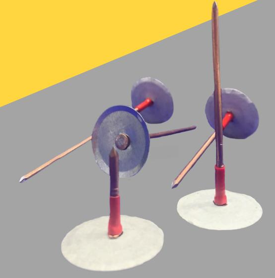
GZONI KP pins are purpose-built for the contact welding of technical insulation onto ventilation ducts and various structures using the "reverse" welding method. These nails feature dual insulation: paper on the washer and PE plastic on the pin. This design prevents burn-through of aluminum foil, and, unlike GZONI nails, they do not require manual application of insulator. This significantly accelerates the installation process.
