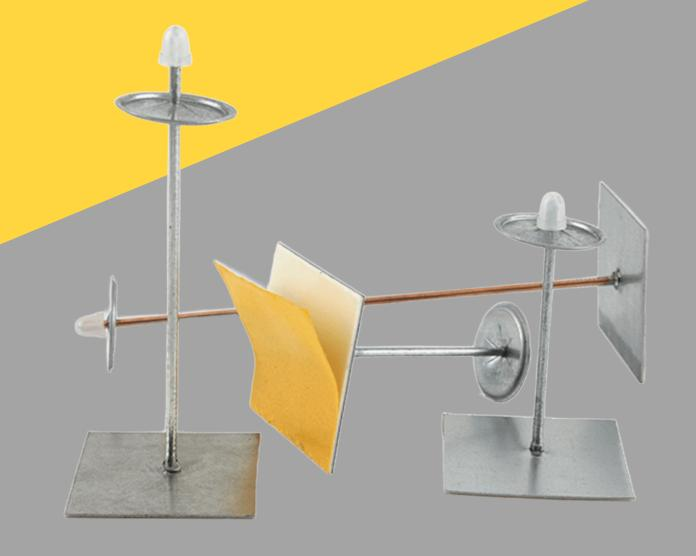
Self-adhesive GSN pins are ideal for the installation of technical insulation on smooth metal surfaces, such as ventilation ducts. These pins feature a square base coated with specialized self-adhesive tape, ensuring a strong and durable attachment. Each set includes a clip and a protective cap, providing a comprehensive solution for secure and aesthetically installation. Their straightforward application and dependable performance make them a versatile choice for various insulation tasks.
